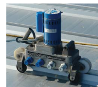
The seaming process uses a heavy-duty four-stand, electric, portable roll-forming machine called the Roof Runner.
